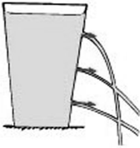
Figure: 2.3 Water pressure acts perpendicular to the sides of a container, and increases with increasing depth.
